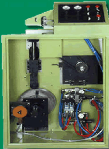
Outboard Cams & Linear Bearings For the Knife Lift
