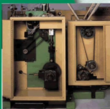
Sideview, without guards, showing linear bearings on hot knife. Also illustrates extensive use of timing belts.
